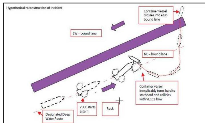
Figure 2: Collision and Oil Spill in Traffic Separation Scheme
